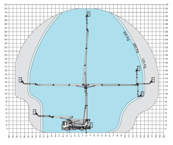
\* outreach and height max values and repeatability can change within ± 3% due to manufacturing variation and working condition.
