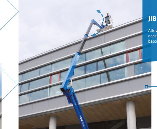
Allows passing over obstacles and to access hard to reach areas, such as balconies, roofs etc.
